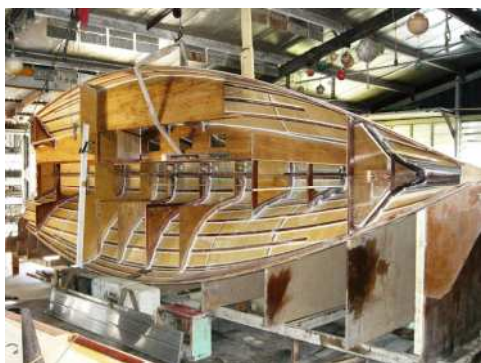
Another way to check bulkhead alignment
