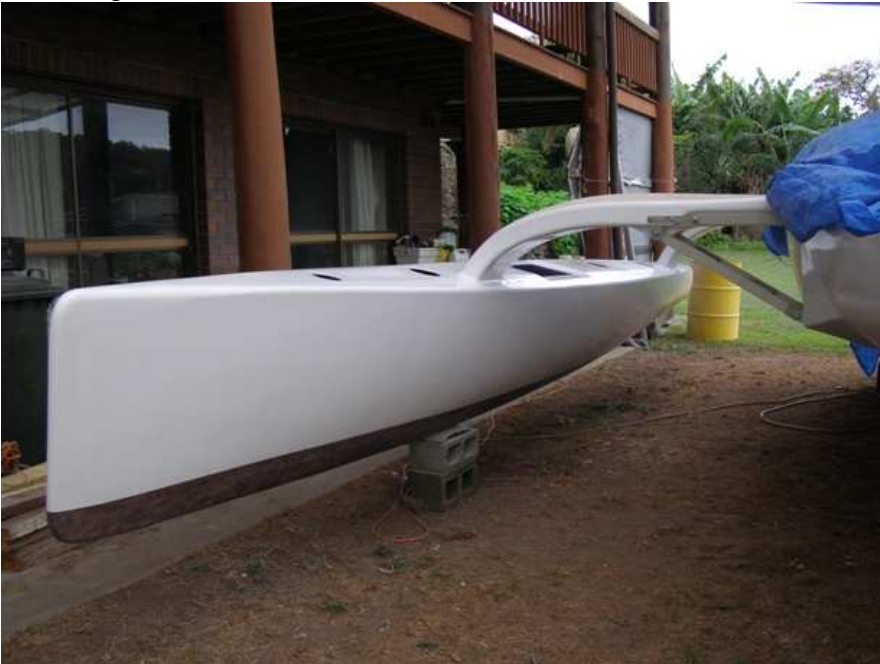
Float decks completed
