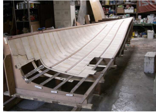
Deck stringers fitted
