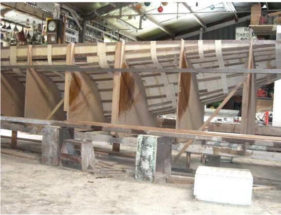
*Main Hull Mould set up – rear view*
