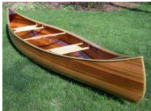
Typical cedar strip plank 'Redbird' canoe
