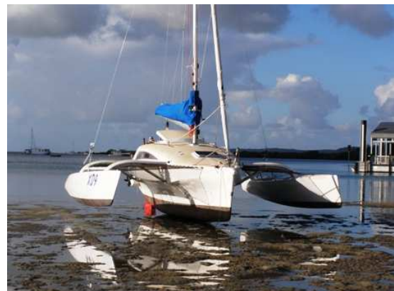
The wavelength dries out on the flat centre hull
