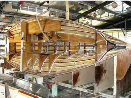
Testing 'fit' of half hulls
