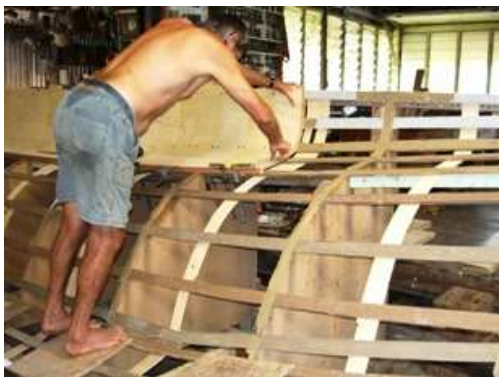
Laminating the main hull
